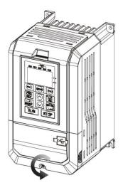
Step 1: Loosen the Screw
