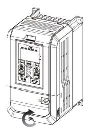
Step 4: Tighten the Screw
