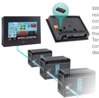
With RS-422/RS-485 communication networks, termination resistors are often required to improve the reliability of communications. External termination resistors can make communication wiring onsite complex. To solve this problem, the P5 provides built-in termination resistor switches. Terminating can be achieved by turning on the switch to connect to termination resistors, or turn off the switch to disconnect the resistors.
